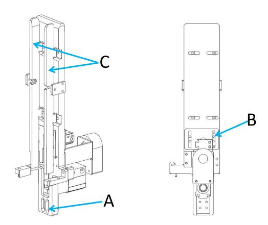
(三): When the length of the tube changes, adjust the back and forth spacing of the vertical plate.
