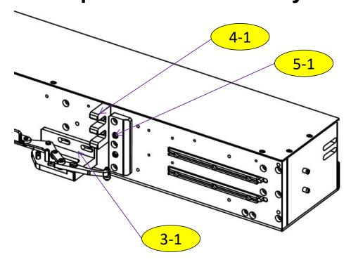
4: When the feeder-lock position lock is not tight: loosen two screws at 3-1 and move forward or backward, so that the round bearing at the front is stuck to the v-groove of feeder-plate 3, which is in contact with the cutting surface, and then tighten the screw.
